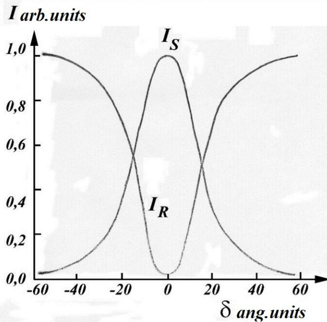
**Fig. 2. Angular dependences of  $I_S$  and  $I_R$  for gratings with 100% diffraction efficiency.**
