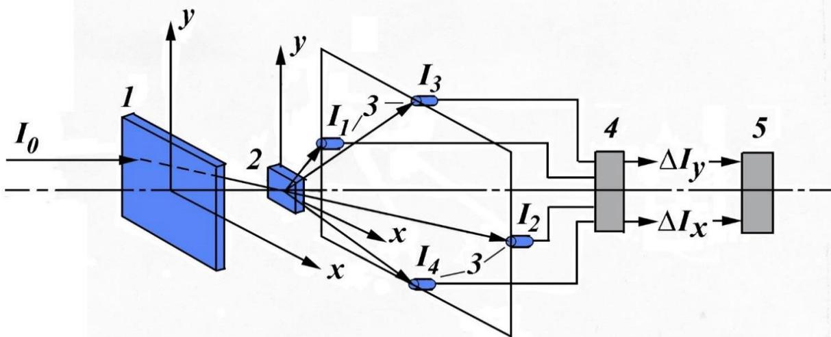
**Fig.12. Schematic diagram of a two-coordinate sensor of the position of a point light source based on GOE: 1 - holographic lens; 2 - GOE, consisting of 4 3D THDG; 3 - photo receivers; 4 - differential amplifier; 5 - indicator device.**
