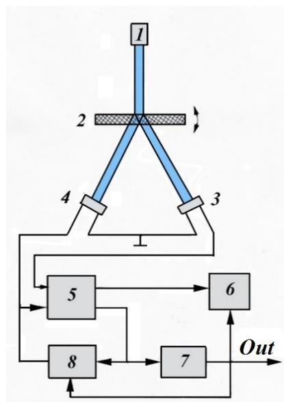
**Fig.6. Schematic diagram of the angle measuring device:** 1 - emitter; 2 – GOE, made in the form of a combination of two 3D THDG, with the same periods and angles of inclination of the stroke planes (Fig.7, a); 3, 4 - photo receivers; 5 – differential amplifier; 6 – display node; 7 – three-stable comparator; 8 - gain control.
