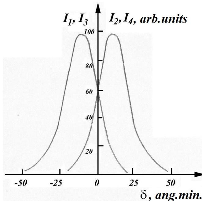
**Fig. 10.** Angular dependence of the intensity of the diffracted beams on the first  $I_1$ , the second  $I_2$ , the third  $I_3$  and the fourth  $I_4$  3D THDG:  $I_1$  ,  $I_2$  – when rotating the GOE relative to the  $Oy$ ;  $I_3$   $I_4$  are relative to the  $Ox$  axis .
