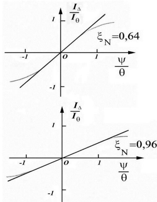
**Fig. 8. Dependence on the angle of incidence of light  $\psi$  normalized to the Bragg angle  $\theta$  on the GOE at different parameters  $\xi_N$ .**
