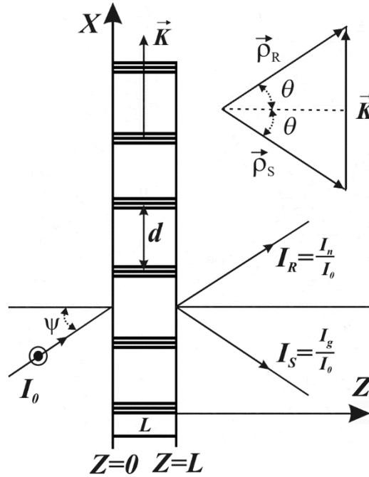
**Fig. 1. Diffraction of monochromatic light on 3D THDG.**
