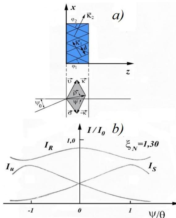
**Fig.7, a) vector diagram explaining the diffraction of light on a combination of two 3D THDGs ; b) dependence of the intensities of the passing beam,  $I_R$  and the diffracted beams  $I_S$  and  $I_u$ , on the angle of light incidence  $\psi$ , which is normalized to the Bragg angle  $\theta$ .**
