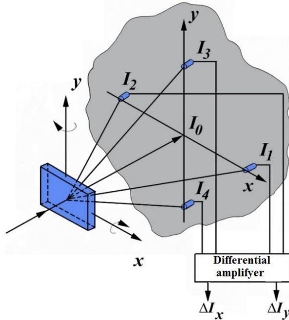
**Fig. 9.** Diffraction of light on GOE (a medium in which four 3D THDGs are recorded):  $I_0$  – a beam of light passing through;  $I_1$  ,  $I_2$  ,  $I_3$  and  $I_4$  are light beams diffracted by 1, 2, 3 and 4 3D THDG, respectively.
