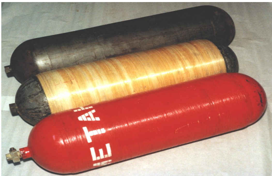
Figure 1 – Test samples of welded metal-plastic cylinders, reinforced with composite material
