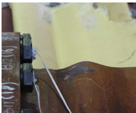
Figure 13 – Local deformation zone of the pipe wall according to experimental data [8]
